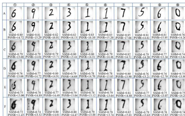
Fig. 4. Visual comparison of the recovery results of different polarization components on the training dataset TR200 over five-fold cross-validation tests using the LGCPFL framework. (A) ground truths; (B) the images recovered by LGCPFL with DoLP; (C) the images recovered by LGCPFL with I_0 ; (D) the images recovered by LGCPFL with I_{45} ; (E) the images recovered by LGCPFL with I_{90} ; (F) the images recovered by LGCPFL with I .
