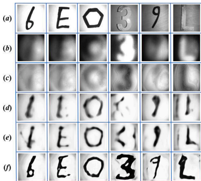
Fig. 12. Visual comparison between the recovery results of PSI-LGCPFL and other methods. (a) ground truths; (b) DCP; (c) Polarimetric-Net; (d) MU-DLU; (e) SAM-MIU-net; (f) PSI-LGCPFL.
